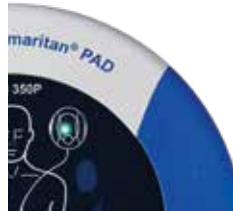
Figure 11. Flashing green LED; no action required.
